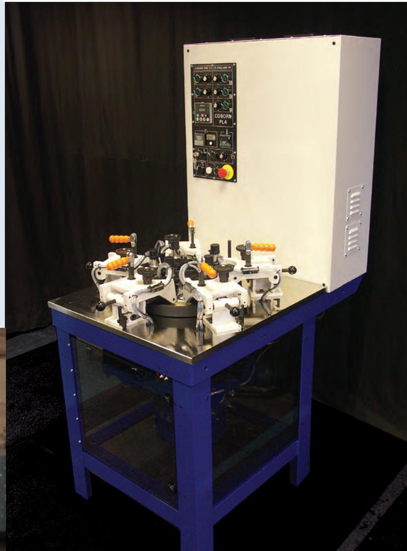
Chilled water is also fed to the back of each disc. This maintains the disc at a uniform temperature to minimise disc dishing.
